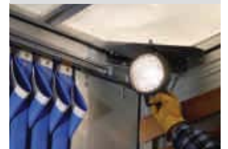
Flush fitting pull-up load anchorage points, 4 per side mounted discreetly into the curtain lower runner section
