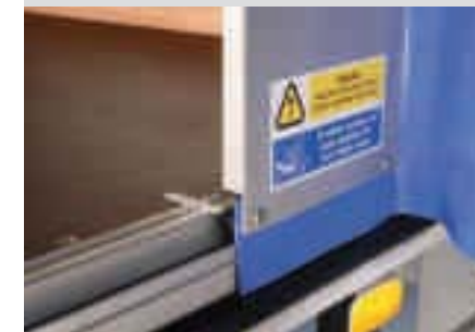
Standard nearside bulkhead mounted grab handle with optional side underrun guard step, tubular stirrup step fitted as standard
