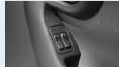
Electrically operated windows.
